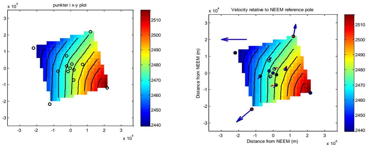
Fig. Left: Map of existing strain net at NEEM. The circles indicate poles. It is of high priority to re-measure the filled poles. The purple circle indicates the reference pole at NEEM. Right: Arrows indicate horizontal surface velocities relative to the NEEM reference pole over the period 2007-2008 (red), 2008-2009 (black), 2009-2010 (blue).
