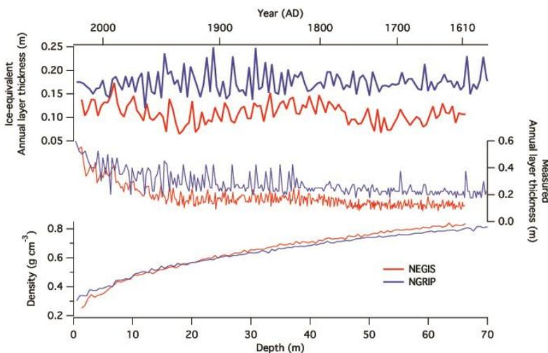
*Reconstruction of the annual layer thickness from the 67 m shallow ice core from NEGIS. The accumulation rate is 0.11 m/yr and a significant increase of accumulation in the more recent warmer years is not observed. The results are compared with records from NGRIP. (P.Vallelonga et al, Preliminary glaciochemical and geophysical study of the Northeast Greenland Ice Stream (NEGIS), submitted to the Cryosphere)*
