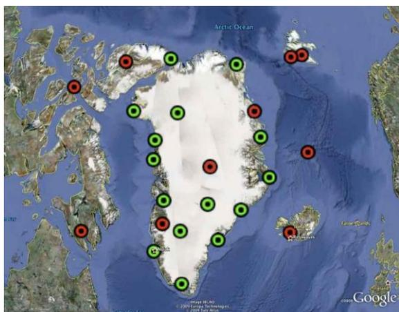
**1** The map shows the location of existing real-time broadband seismic stations (red) joining GLISN with open data sharing and sites (green) where equipment, telemetry, and infrastructure is being installed and upgraded in concert with GLISN partners.
