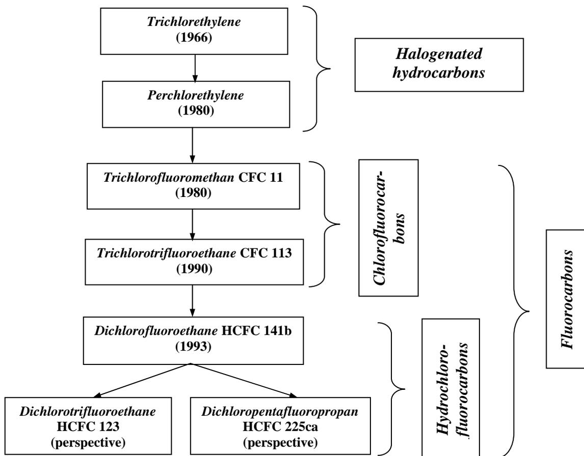
*Fig.1. Densifiers for ice deep drilling (in brackets: the year of first use)*
