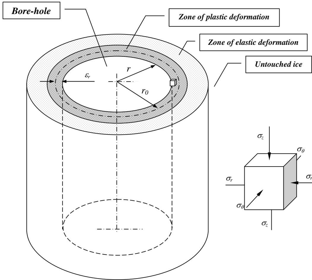
**Fig. 2. Deformation of ice near the bore-hole ( $r_0$  – initial radius;  $r$  – current radius)**
