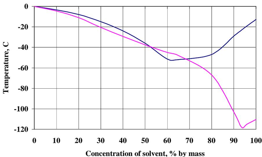
— Aqueous solution of ethylene glycol — Aqueous solution of ethanol
