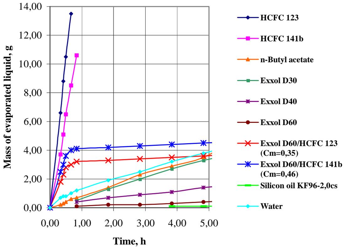
**Fig.3. Vaporization rate of solvent Exxol D60 and silicon oil KF96-2,0cs**
