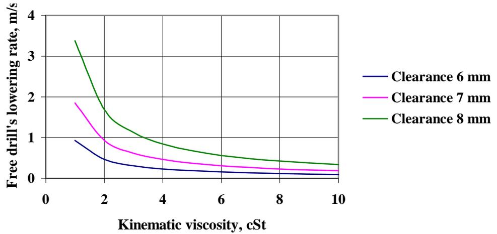
**Table 2. Free drill's lowering rate versus kinematic viscosity of the hole fluid**
